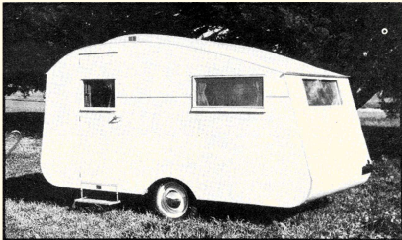
Note the English-style gable roof, long since discontinued in Australia, that was popular at the time this early ply van was built. It would weigh as much as an eighteen footer today, since the earliest vans were built of quite heavy materials.
