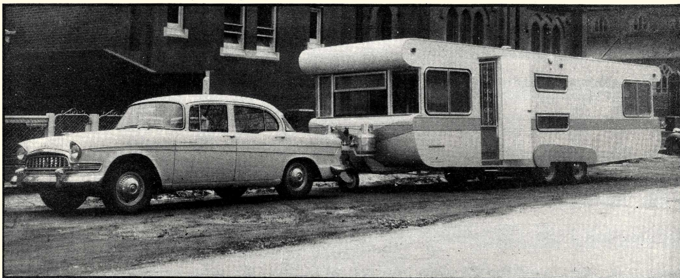
Twenty five years ago Franklin was (and still is) a most important name in caravan construction. Bondwood and marine ply was the standard form of wall construction before aluminium sheeting became so popular.
