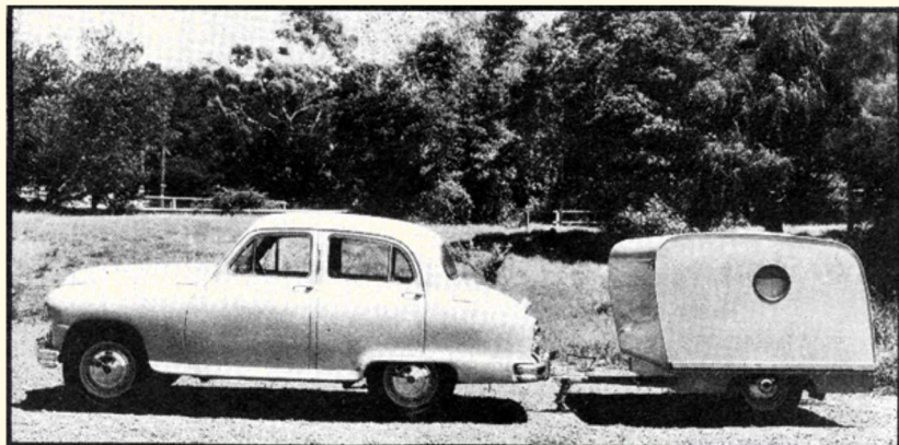
Invented by a Sydney resident in the Forties and patented so that no one was ever able to copy his design, this Proper plywood camper was small and easy to tow on the road and opened up to twice its towing size on site. Obviously the first of the expanding campers. Very soundly built, these units are still giving good service in many parts of Australia.
